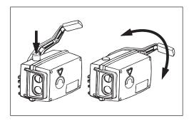
When placing the actuator in manual operation power should be turned off to the actuator. In the event the actuator is powered and is left in a manual position, the result could lead to the internal damage of the actuator.
